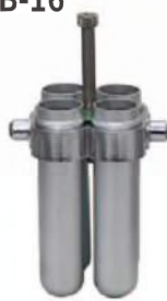
15ml×4tubes, 17×88mm, 4,500RPM, 3,736xg
